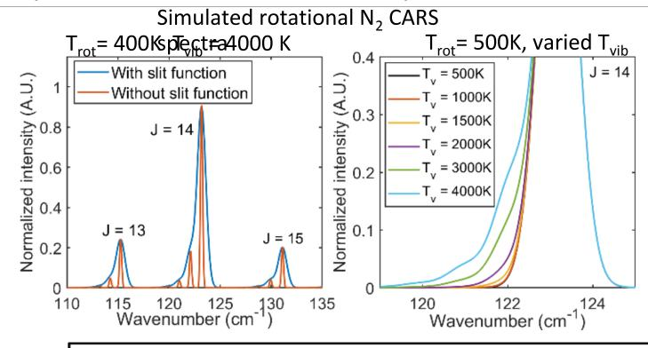
Increasing vibrational energy level red-shifts the rotational energy level F(v,J)
